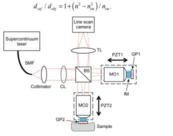
Fig. 1. Schematic of the LC-OCT system. TL: tube lens; PZT: piezoelectric actuator; MO: microscope objective; IM: immersion medium; SMF: single mode fiber; BS: beam-splitter; CL: cylindrical lens. GP: glass plate. The plain red lines represent the beam in the plane of the figure (the cylindrical lens has no effect in this plane). The dotted red lines represent the beam in the direction orthogonal to the plane of the figure.
