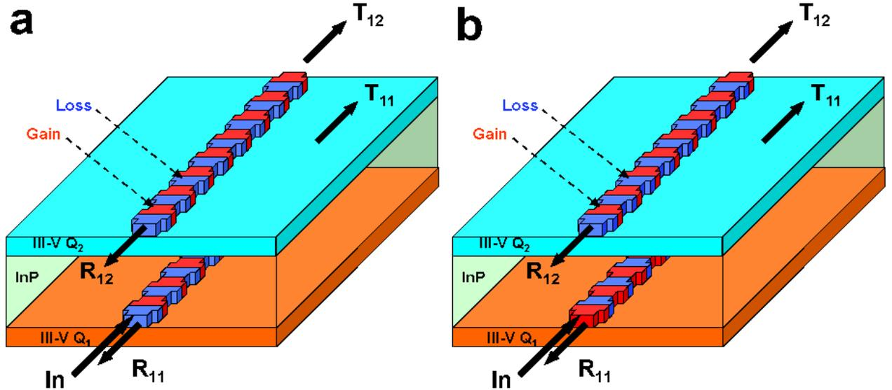
Figure 4. Sketch of a PTSBG assisted directional coupler with rectangular grating profile. Gain and loss grating sections are indicated by red and blue colors, respectively: a) Symmetric gain/loss index profile distribution between top and bottom waveguides; b) Anti-symmetric gain/loss index profile distribution between top and bottom waveguides.
