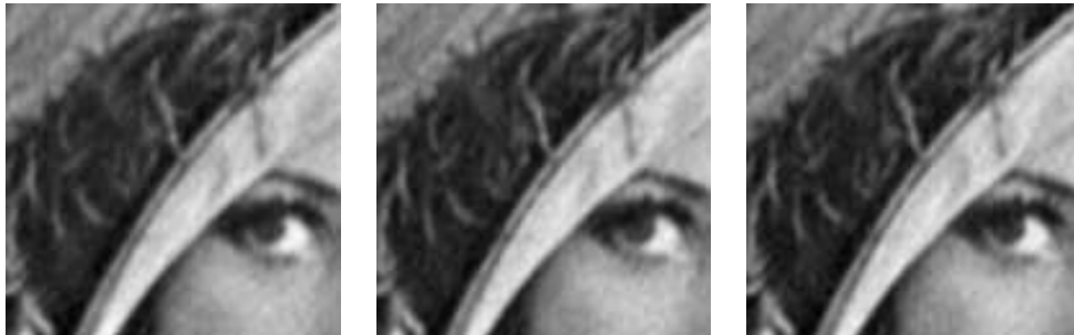
Fig 13 Image and zoom-ins of Lena obtained for defocus \psi = \psi_{max} with the simulated hybrid imaging system with masks optimized for \psi_{max} = 2.0\lambda and different numbers of rings.
