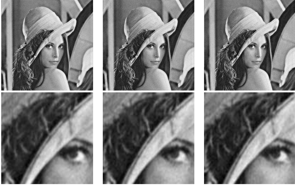
Fig 13 Image and zoom-ins of Lena obtained for defocus \psi = \psi_{max} with the simulated hybrid imaging system with masks optimized for \psi_{max} = 2.0\lambda and different numbers of rings.
