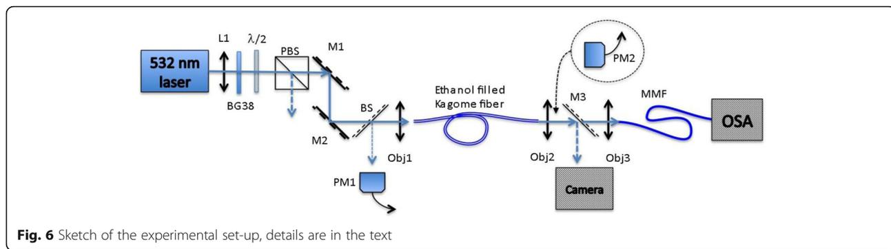
Fig. 6 Sketch of the experimental set-up, details are in the text
