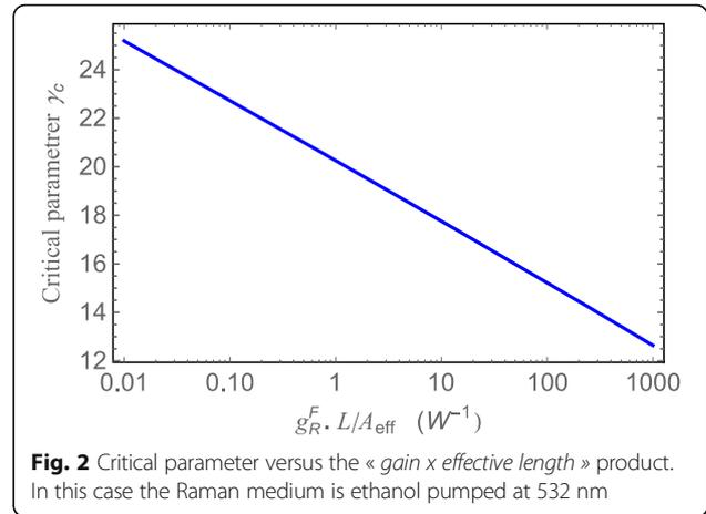
thumb rule to start designing a Raman converter is to state that  $\gamma_C \approx 20$ . We can also express this feature in terms of pump power required to reach the critical parameter,  $P = \gamma_C A_{eff}^R / (g_R^f L)$ : increasing the fiber length by a factor  $10^5$  and decreasing the pump power by a factor  $2 \times 10^5$  allows keeping the same Raman conversion efficiency.
