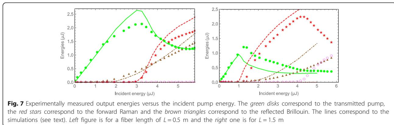
Fig. 7 Experimentally measured output energies versus the incident pump energy. The green disks correspond to the transmitted pump, the red stars correspond to the forward Raman and the brown triangles correspond to the reflected Brillouin. The lines correspond to the simulations (see text). Left figure is for a fiber length of  $L = 0.5 \text{ m}$  and the right one is for  $L = 1.5 \text{ m}$
