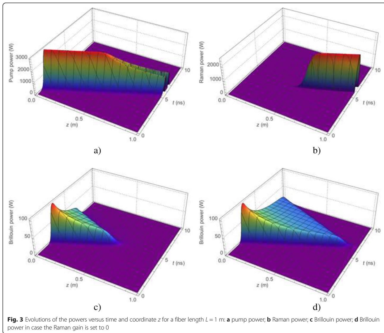
**Fig. 3** Evolutions of the powers versus time and coordinate  $z$  for a fiber length  $L = 1$  m: **a** pump power; **b** Raman power; **c** Brillouin power; **d** Brillouin power in case the Raman gain is set to 0
