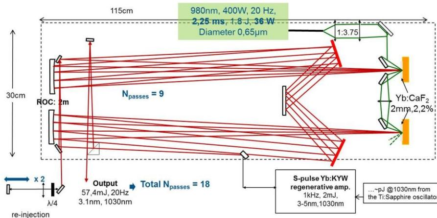
Figure 1: Multipass amplifier setup using 2 Yb-CaF<sub>2</sub> active-mirror crystals. For clarity only 4 passes have been represented.
