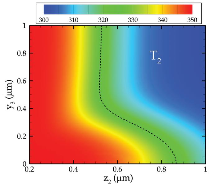
FIG. 3. (Color online) Equilibrium temperature of particle 2 when the three particles have coordinates  $\mathbf{R}_1 = (0, 0, 0)$ ,  $\mathbf{R}_2 = (0, 0, z_2)$ , and  $\mathbf{R}_3 = (0, y_3, z_2/2)$ . Particle 1 is kept at a temperature  $T_1 = 350$  K and the bath has a temperature  $T_b = 300$  K. The black dashed line corresponds to  $T_2 = 325$  K.
