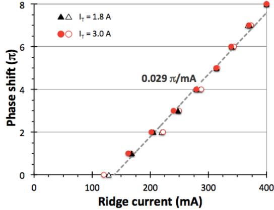
Figure 3: Shift of the fringe pattern as a function of the ridge current for a tapered amplifier, measured at the taper currents  $I_T = 1.8$  A (black triangles) and  $3.0$  A (red circles) and for two different injected optical powers  $P_{in} = 1.5$  mW (empty) and  $P_{in} = 10$  mW (full)
