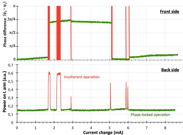
Figure 7: (bottom) Evolution of the power on the L arm (back side) as a function of the current change in one laser for  $I_1 \cong I_2 \cong 140$  mA; the two lasers are phase-locked when the losses L are minimum – green zone of the graph; (top) Evolution of the phase difference on the front side, measured during the same current change.
