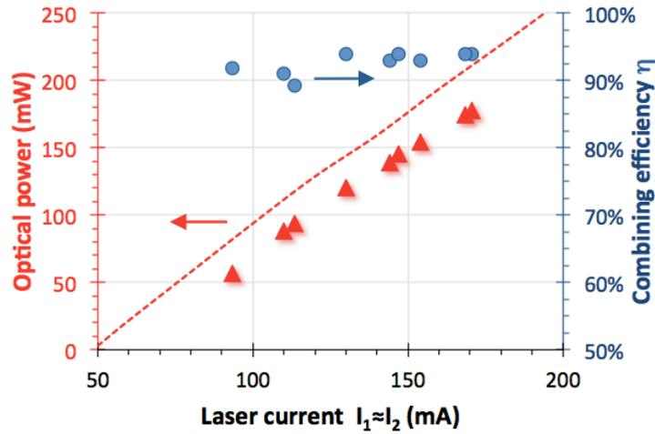
Figure 6: Coherently combined power (red triangles) and combining efficiency  $\eta$  (blue circles) as a function of the operating current of the two lasers; the red line corresponds to the sum of the output powers extracted from each laser independently.
