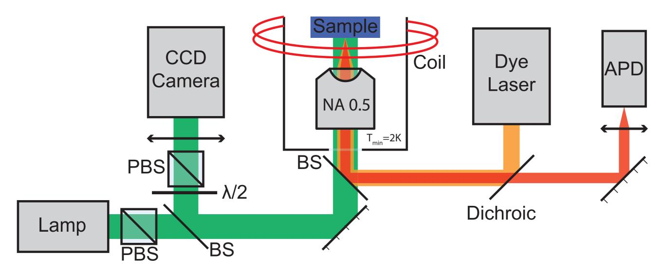
MO imaging setup combined to Single Molecule Spectroscopy
