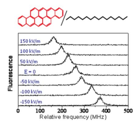
$\Delta E \sim 10 \text{ kV/m}$  will shift ZPL by  $\sim 20 \text{ MHz}$
