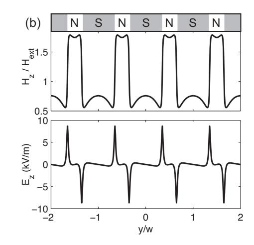
$$H_n(z) = -\frac{2H_{\text{ext}}}{q_n d_N} \left( 1 - e^{-q_n D} \right) e^{-q_n z} \sin \left( \frac{q_n d_S}{2} \right)$$
