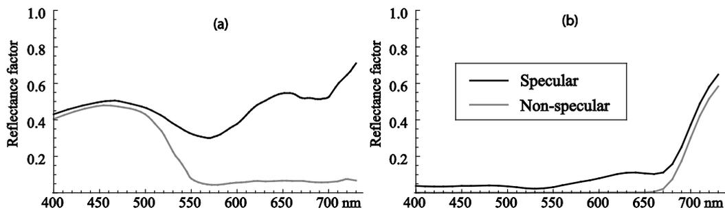
Fig. 4. Spectral reflectance factors of (a) cyan inkjet ink and (b) black ballpoint pen ink on glossy white paper, measured in steps of 10 nm in a  $45^\circ:45^\circ$  geometry (black lines) or a  $35^\circ:45^\circ$  geometry (grey lines).
