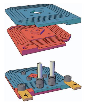
FIG. 3. Assembly of the two coils (top) to form the final magnet (bottom). The artist's view of the magnet also shows the tightening screws, the electric connections, and the quick release hydraulic couplings with related tubes (Rilsan<sup>®</sup>; outer  $\phi = 6$  mm, inner  $\phi = 4$  mm).
