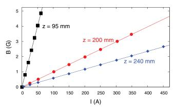
FIG. 6. Axial component of the magnetic field measured by the magnetoresistive magnetometer as a function of the current. Three different graphs are plotted, each corresponding to a different position z of the sensor with respect to the magnet. The best-fit straight lines to the points are also shown. For the last two positions, the AC power supply (50 Hz) was used, and the reported current and magnetic field values are rms.
