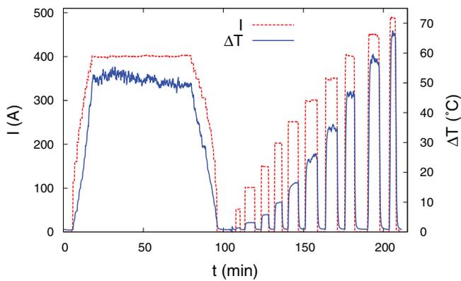
FIG. 7. Magnet temperature increase (blue, solid line), with respect to the pipe temperature ( $\approx 13 \pm 1$ ) °C, as a function of time and in case of a varying current (red, dashed line) flowing through the magnet. During the first 100 min of *normal operation*, the water flux was 1.2 l/min; during the last 100 min of *stress test*, the water flux was 1.3 l/min. All measurements reported in this figure were carried out by using the AC power supply (50 Hz); the current values are rms.
