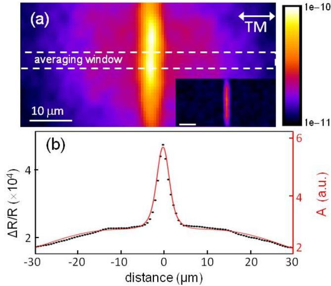
**FIG. 2.** Thermoreflectance data for a 300-nm-width slit. (a) Images obtained for TM polarization (the inset is obtained for TE). (b) Data (black dots) are obtained by averaging 40 line scans from (a). The solid red curve represents the calculated absorption profile  $A(x)$  convoluted by a Gaussian with a FWHM equal to the waist ( $2.8 \mu\text{m}$ ) of the probe beam.
