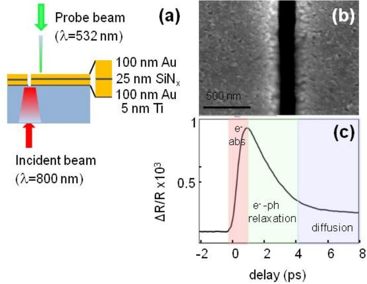
**FIG. 1** (a) Sketch of the sub-picosecond pump-probe slit-experiment. The inset shows the multilayer structure of the sample. (b) Scanning Electron microscope image of the slit used in the experiment. (c) Time-resolved response of a 200-nm-thick gold layer as a function of the pump-probe delay.
