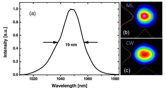
Fig. 2. (a) Spectrum measurement. Far-field spatial beam in (b) ML and (c) CW regime.
