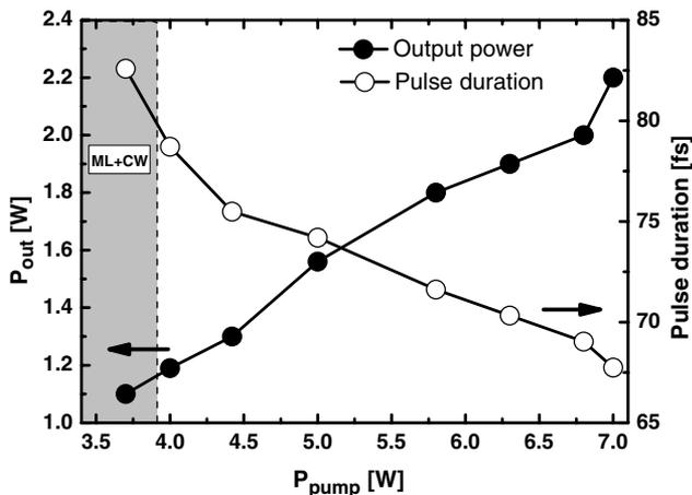
Fig. 4. Output power and pulse duration of the ML Yb:CaF<sub>2</sub> oscillator as a function of the pump power.
