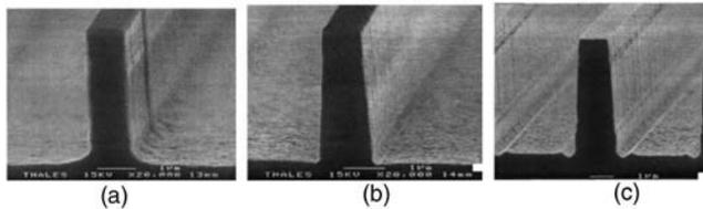
FIG. 5. SEM pictures for the etched ridge waveguides with  $P_c$  varied over (a) 300 W, (b) 600 W, and (c) 900 W, respectively. The platen power is fixed at 150 W. The etch profile shows a transition between an etch foot and a trench with coil power variation.
