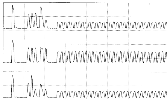
Fig. 8. Output signals obtained by the simultaneous self-routing operation of three channels of the setup. We recorded the three traces one after the other by moving the single-channel receiver into the different output beams. The packet is addressed to output 59 and the three observed outputs are channels 63, 59, and 47.
