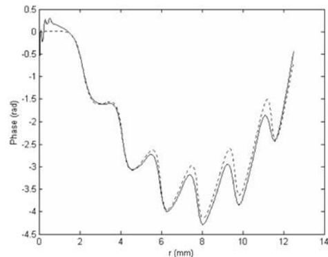
Fig. 2. Phase profiles of the phase mirror: specification (solid curve), interferometric measurement (dashed curve). The phase versus radius  $r$  is given without curvature ( $R = 6$  m), and  $r = 0$  is the mode center.
