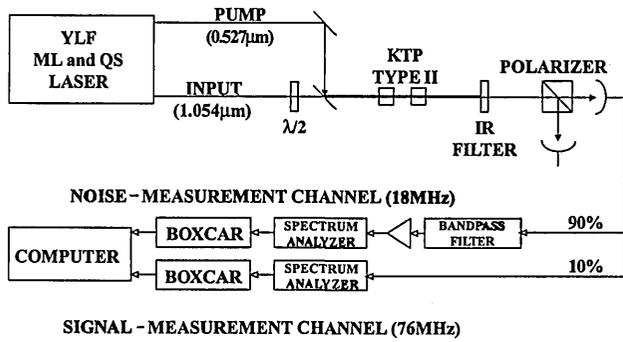
Fig. 2. Experimental setup. A frequency-doubled mode-locked (ML)  $Q$ -switched (QS) YLF:Nd laser pumps (at 527 nm) a traveling-wave parametric amplifier composed of two type-II KTP crystals. The polarization of the input signal (at 1054 nm) is rotated by the half-wavelength plate ( $\lambda/2$ ) to achieve phase-insensitive or phase-sensitive amplification. The photodiode current is split 90/10, with each partial current measured by use of a spectrum analyzer and a boxcar combination.
