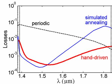
Fig. 7. Radiation loss spectra  $L = 1-R$  for air-bridge mirrors with two-segment tapers. Red bold curve: hand-driven design for segments defined by  $(a', d) = (320, 170)$  nm, and  $(a'', d) = (280, 100)$  nm. Blue thin curve: optimized design for segments defined by  $(a', d) = (240, 210)$  nm, and  $(a'', d) = (414, 100)$  nm. The dashed curve corresponds to the modal reflectivity of the periodic mirror and the vertical dotted lines indicate the band edge.
