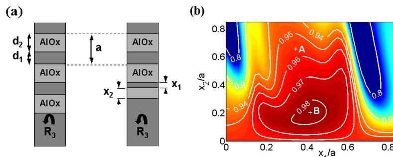
Fig. 6. Single-segment tapers for micropillar Bragg reflectors. (a) Reflector geometry ( $a = d_1 + d_2 = 228 \text{ nm}$ ). Dark and light regions correspond to GaAs and AlO<sub>x</sub> materials. (b) Modal reflectivity as a function of the normalized thicknesses  $x_1/a$  and  $x_2/a$  of the first GaAs and AlO<sub>x</sub> layers for  $\lambda = 0.95 \mu\text{m}$ . Points A and B correspond to geometries with periodic and optimized mirrors, respectively.
