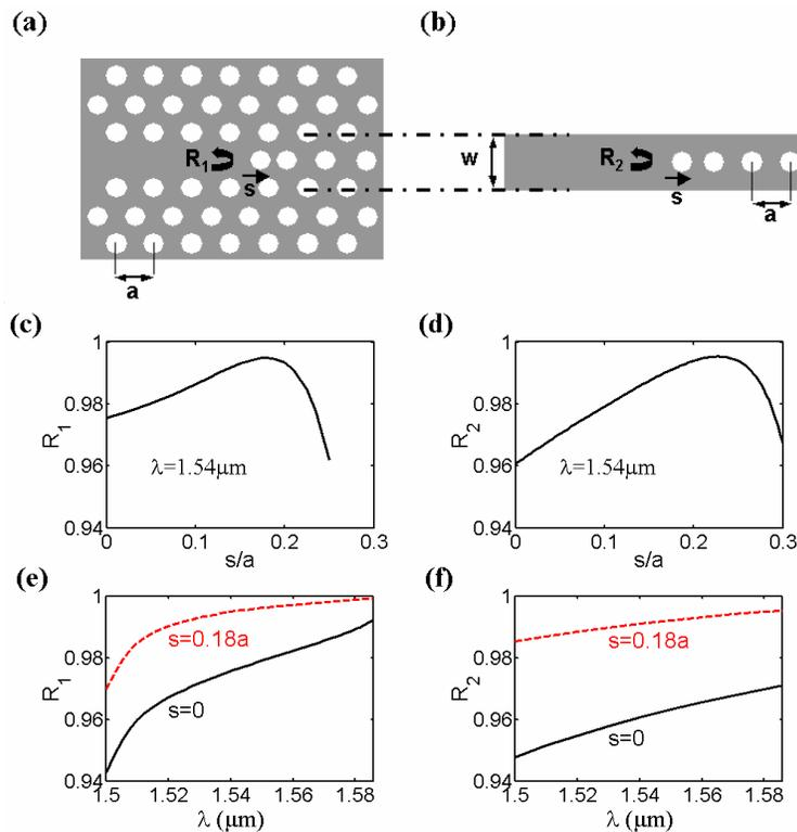
Fig. 5. Effect of hole shifting on the modal reflectivity of 1D and 2D PC mirrors. (a) 2D PC configuration. (b) Related air-bridge configuration. (c) and (d) Modal reflectivities  $R_1$  and  $R_2$  for  $\lambda = 1.54 \mu\text{m}$  as a function of the normalized hole shift  $s/a$ . (e) and (f) Corresponding modal reflectivity spectra. The solid and dashed curves are obtained for  $s = 0$  and  $s = 0.18a$ , respectively.
