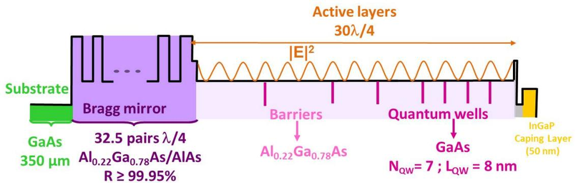
Figure 1: Semiconductor structure design.
