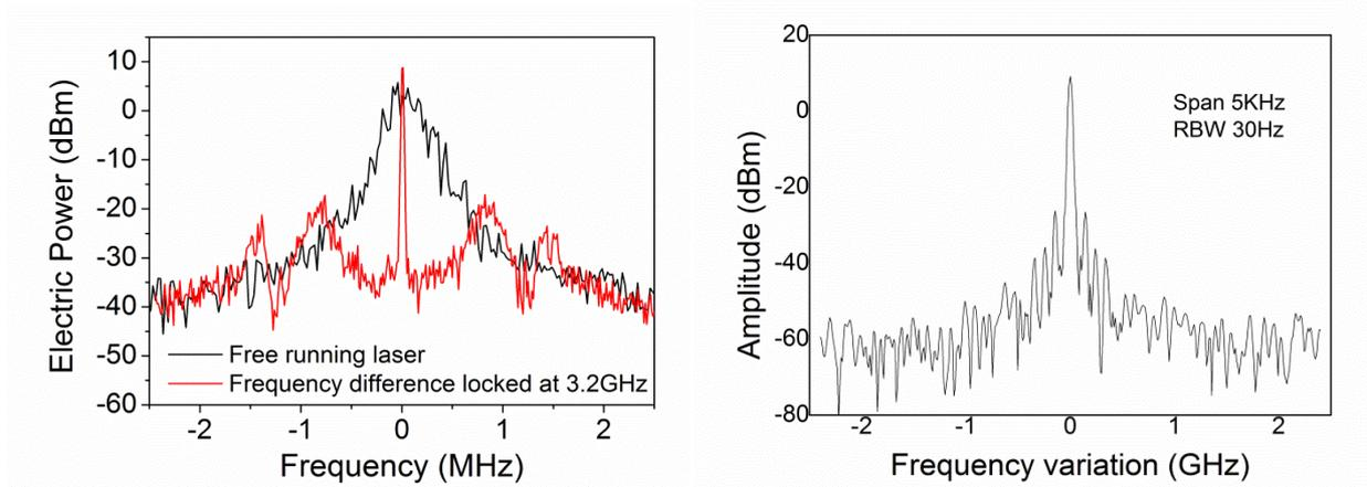
Figure 9: *Left:* Beat note of the free running laser and the frequency difference locked at the RF reference at 3.2GHz. *Right:* Beat note spectrum of the locked laser with a span of 5KHz.
