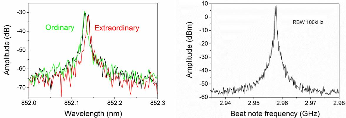
Figure 5 : *Left*: High-resolution optical spectrum of the 2-frequency laser around 852.1nm (resolution = 2 pm). *Right*: Beat note frequency around 3GHz.
