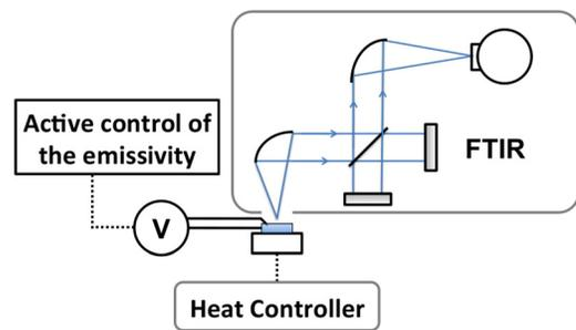
FIG. 2. Experimental setup used to characterize the modulated thermal emission of the structure. The temperature of the sample is set to  $70^\circ\text{C}$ . A DC gate voltage ranging from  $-400\ \text{mV}$  to  $400\ \text{mV}$  is applied and allows an active control of the emissivity. The radiation is spectrally analyzed using an infrared Fourier transform spectrometer (FTIR) with a mylar beamsplitter and a DTGS detector.
