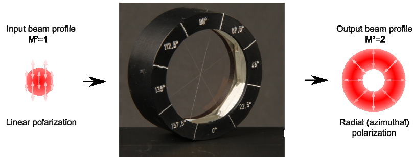
Fig. 3. Linear to radial / azimuthal polarization converter based on segmented waveplates. The lowest transversal order mode with cylindrical polarization is the LG_{01}^* -mode with a donut-shaped intensity distribution.
