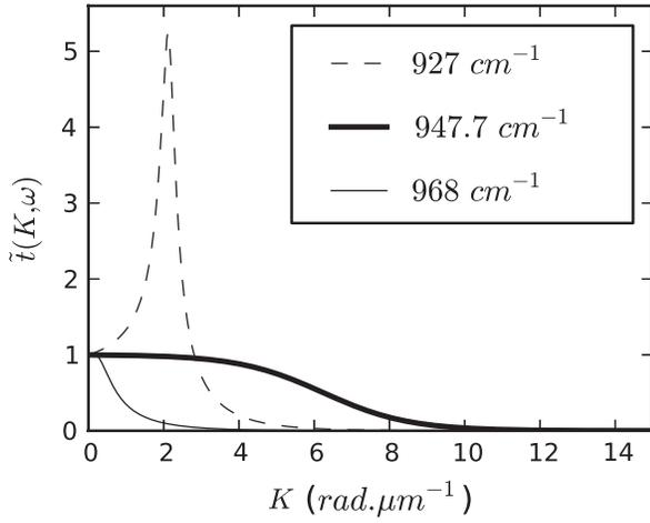
FIG. 3. Transmission factor as a function of the wave vector for three different frequencies. An ideal superlens is characterized by a transmission factor  $\tilde{t}(K, \omega) = 1$  at the optimum frequency. In the presence of losses, we obtain the best behavior at  $\omega = \text{Re}(\omega_{\text{sw}})$ .
