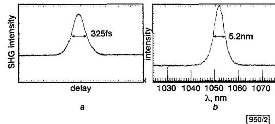
Fig. 2 Temporal and spectral characteristics of 210 fs pulses
