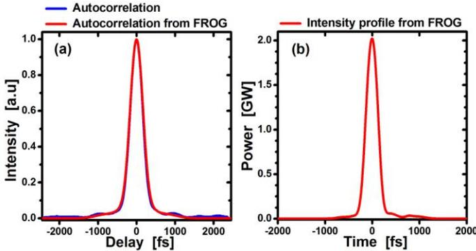
Figure 3: (Color online) (a) Autocorrelation traces measured at 650  $\mu\text{J}$  (blue) with an independent autocorrelator and (red) from a FROG measurement. (b) Retrieved temporal profile of the pulse from the FROG measurement (Error  $27.10^{-4}$  on a  $256 \times 256$  grid).
