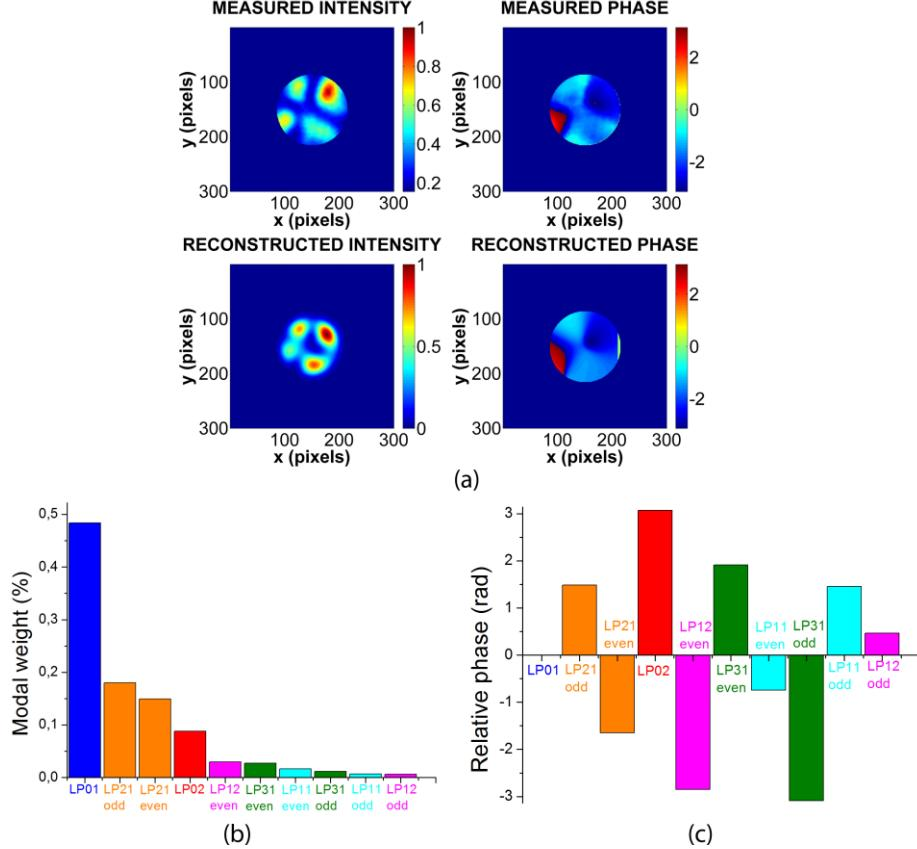
Fig. 6. (a). Measured and reconstructed phase and intensity profile in the case of an excitation close to the  $LP_{21}$  mode. The intensity profile is normalized and the phase is given between  $[-\pi, \pi]$ . (b) and (c): Corresponding modal decomposition.
