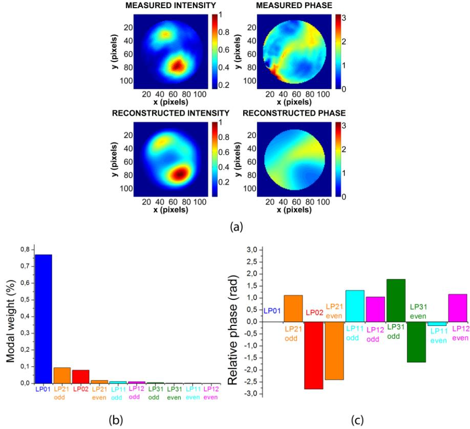
Fig. 7. (a). Measured and reconstructed phase and intensity profile in the case of an arbitrary mode excitation. The intensity profile is normalized and the phase is given between  $[0, \pi]$ . (b) and (c): Corresponding modal decomposition.
