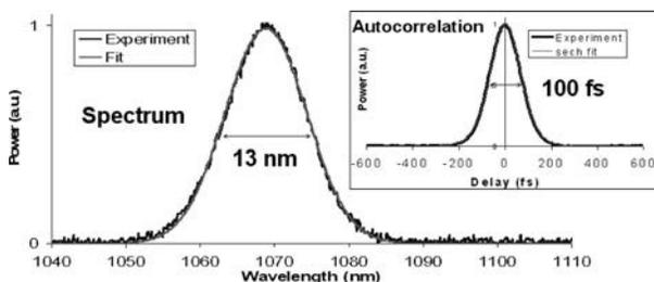
Fig. 4. Spectrum and autocorrelation traces of 100-fs pulses.
