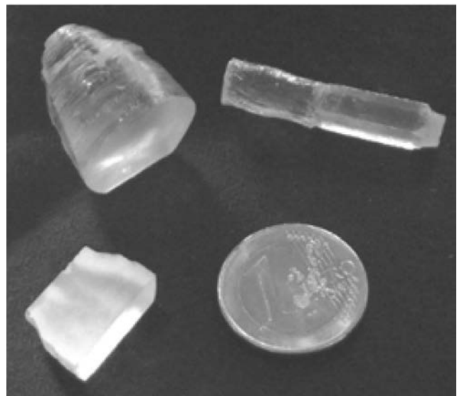
Fig. 3. Several pieces of 5.5%-doped Yb:SYS, along with a 1 Euro coin for scale.
