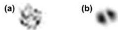
Fig. 3. Beam shapes: (a) incident pump beam; (b) reflected Stokes beam (LP 11 mode).
