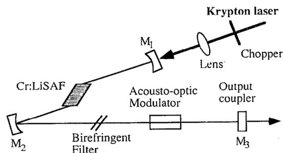
FIG. 1. Experimental set-up M<sub>1</sub> and M<sub>2</sub> are R=100 mm HR mirrors. M<sub>3</sub> is a plane mirror with a transmission of 22.5%.
