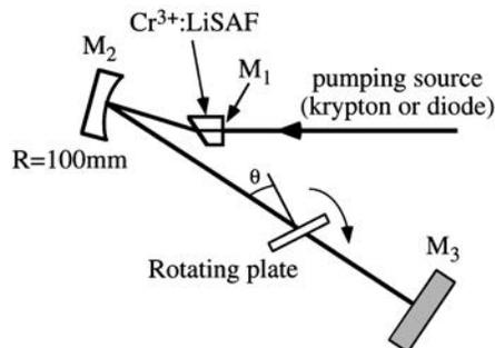
Fig. 1. Experimental setup for small-signal gain measurement.
