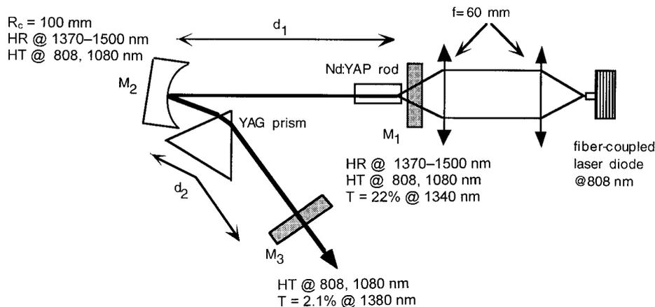
Fig. 1. Diode-pumped Nd:YAlO<sub>3</sub> laser operating on the 1378- and 1385-nm lines.
