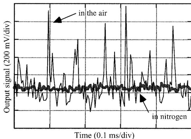
Fig. 2. Output signals for a Nd:YAlO<sub>3</sub> laser on the 1378- and 1385-nm lines operating in the air (thin curve) and in an atmosphere purged of water vapor (thick curve).
