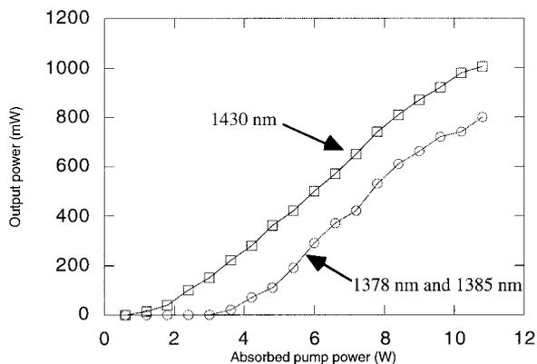
Fig. 3. Output power versus absorbed pump power for a Nd:YAlO<sub>3</sub> laser: comparison between the 1378- and 1385-nm lines (circles) and the 1430-nm line (squares).
