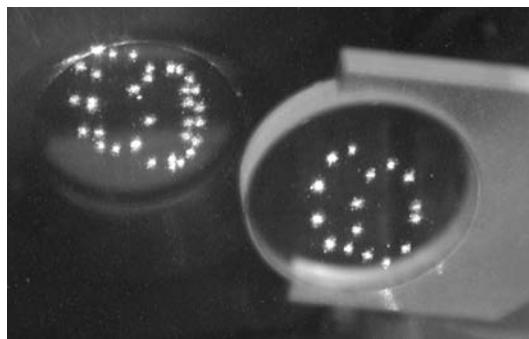
Fig. 2. Photograph of the MPC concave mirrors with the beam spot pattern on them for the 1.2-MHz repetition-rate mode-locked Nd:YVO 4 laser.
