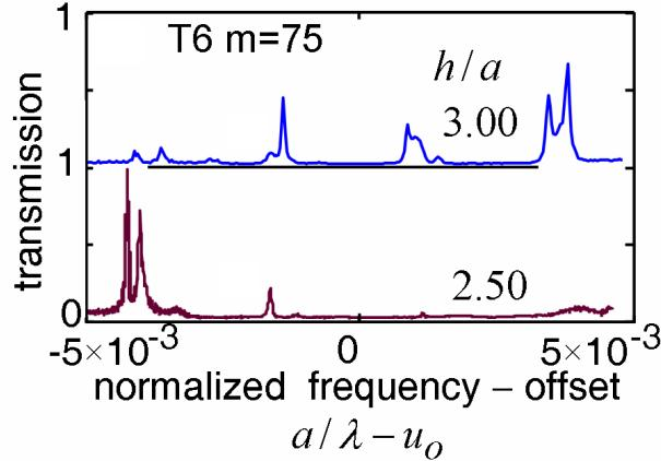
Figure 4. Experimental spectra for waveguides of order  $m = 75$ , of length "T6" (see Fig.2) and of height/period ratio  $h/a = 3.00$  and  $2.50$  as indicated. Note the doublets for  $h/a = 3.00$  which become more markedly singlet-type for the more exact CCR condition  $h/a = 2.50$ .
