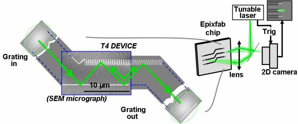
Figure 3. Sketch of a typical EpixFab chip/sample and of optical setup to measure it with a tunable laser triggering the camera.
