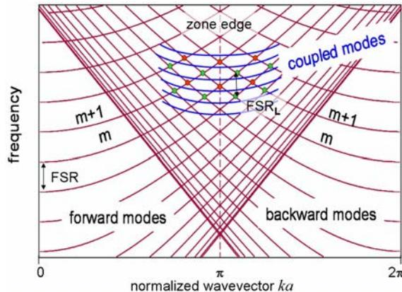
Figure 1. Crossing of forward and backward modes in an ideal broad waveguide (half-hyperbola) form a nearly regular mesh (dots). The corrugation can couple these modes and form hyperbola of “slow modes” centered at the band edge  $ka=\pi$ .
