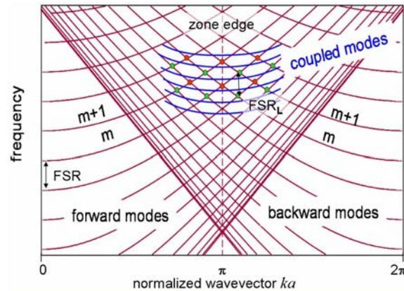
Figure 1. Crossing of forward and backward modes in an ideal broad waveguide without corrugation (half-hyperbola) form a nearly regular mesh (dots). The corrugation can couple these modes and form hyperbola of "slow modes" centered at the band edge  $ka=\pi$ .
