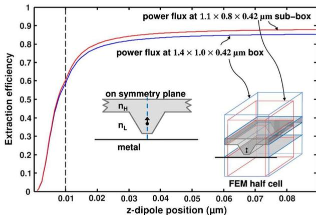
Fig. 8. (Color online) Light capture efficiency by a PIROW on both sides for a dipole lying along the vertical direction at  $x = 0$ . Insets show (left) the scanned position and the nominal and (right) the two “nested” collection boxes used to check that extraction is in the far-field regime.
