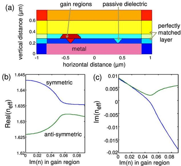
Fig. 9. (Color online) (a) Map of coupled PIROW guides with attempt to implement PT symmetry onto the left one with the same variable added gain  $g$  in the inverse ridge and in the shaded region above it, (b) real part of  $n_{\text{eff}}$ , and (c) imaginary part of  $n_{\text{eff}}$
