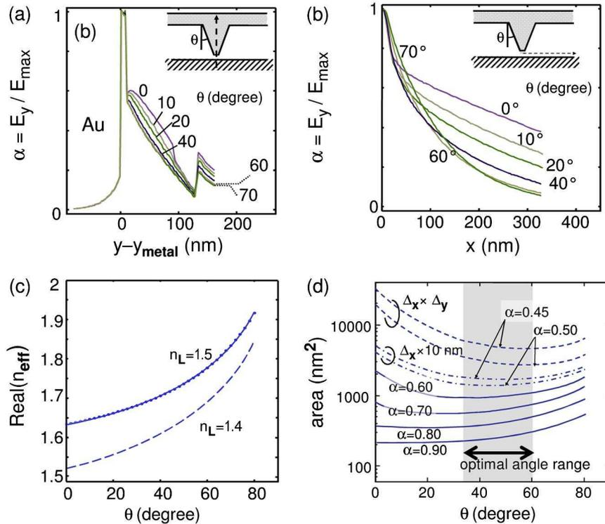
Fig. 2. (Color online) PIROW modal characteristics for tip width  $L_{\text{tip}} = 20$  nm,  $n_L = 1.40$ , and variable inverse-rib angle  $\theta$ . (a), (b) Field profiles along the cuts indicated in their inset. (c)  $(\text{Re}(n_{\text{eff}}))$  trend versus angle  $\theta$  (dashed line), with comparison to  $n_L = 1.50$  (solid line with dots). (d) Area enclosed in the range  $|E_y| > \alpha E_y^{\text{max}}$  versus angle for different values of  $\alpha$ .
