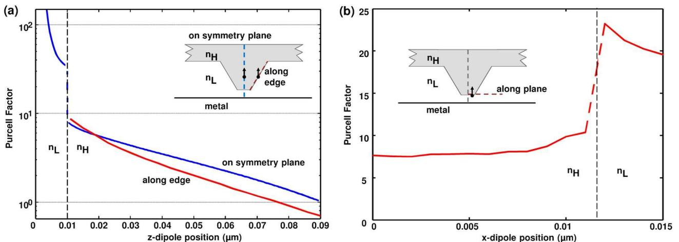
Fig. 7. (Color online) Purcell factor  $F_p$  for a vertical dipole at wavelength  $\lambda = 700$  nm in a PIROW: (a) dipole at variable height, either in the symmetry plane  $x = 0$  or along the rib edge and (b) dipole lying along  $x$  at height  $z = d$ , the height of the tip bottom. Insets, scanned positions.
