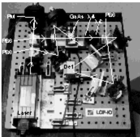
Figure 6 : Photo of the experimental set-up used in the study, with the beams indicated. PBS : polarizing beam splitter, PM piezomirror,  $\lambda/4$  : quarter wave plate,  $\lambda/2$  : half wave plate, Det : differential detector.
