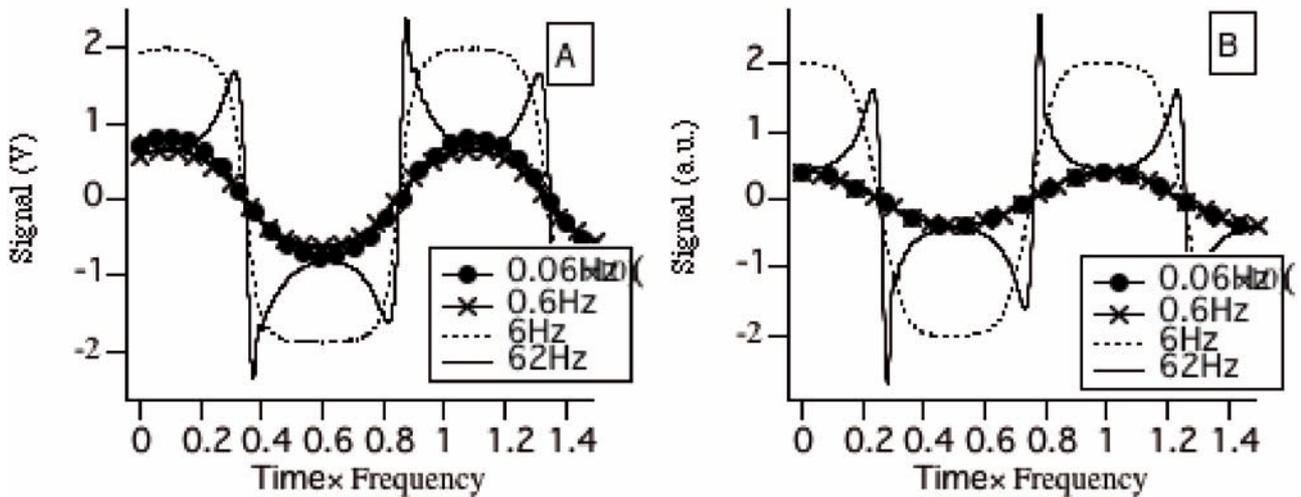
Figure 8 : Experimental response (A) of the photorefractive velocimeter to a sinusoidal phase modulation of fixed amplitude ( $11.4\mu\text{m}$ , except for the  $62\text{Hz}$  signal corresponding to a  $9.9\mu\text{m}$  displacement amplitude) having an increasing frequency. In (B) are shown the calculated responses of the photorefractive velocimeter.
