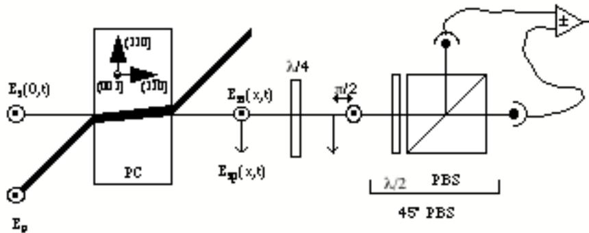
Figure 1 : Scheme of a photorefractive beam combiner based on the anisotropic diffraction configuration. PBS is a polarizing beam splitter, PC is the photorefractive crystal,  $\lambda/2$  and  $\lambda/4$  are half and quarter wave plates respectively.
