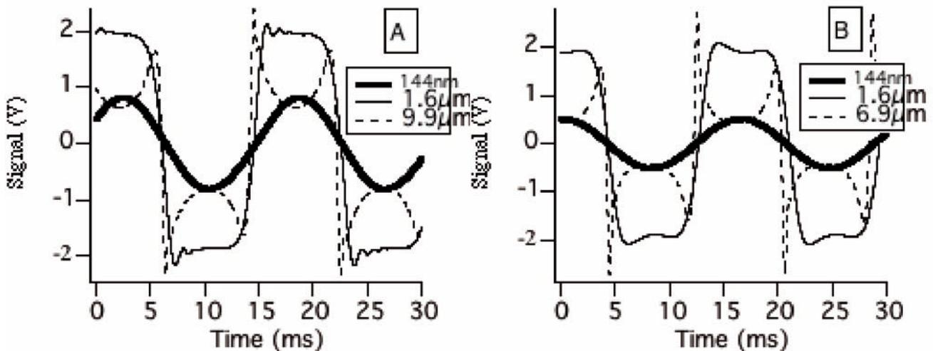
Figure 9 : Experimental response (A) of the photorefractive velocimeter to a sinusoidal phase modulation of fixed frequency ( $60\text{Hz}$ ) and of increasing amplitude. In (B) are shown the calculated responses of the photorefractive velocimeter.
