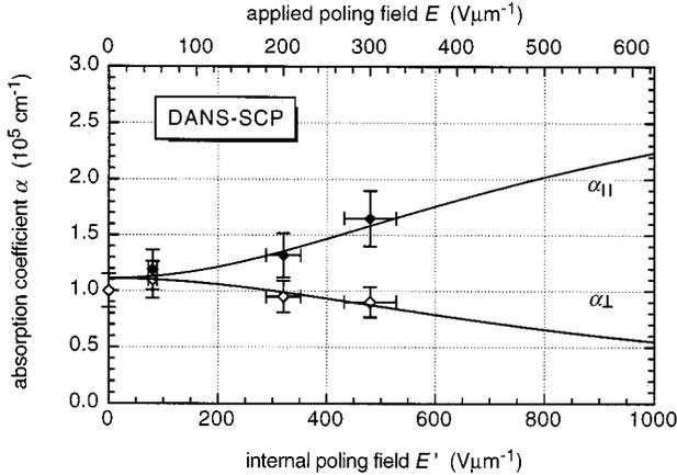
Fig. 6. Poling field dependence of the absorption coefficient for polarization parallel ( $\alpha_{\parallel}$ , filled diamonds) and perpendicular ( $\alpha_{\perp}$ , open diamonds) to the poling field, measured on in-plane poled DANS-SCP samples at a wavelength of  $0.458 \mu\text{m}$ ; curves, fits to Eqs. (12) and (13), respectively.
