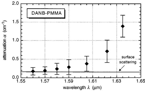
Fig. 5. Attenuation coefficient  $\alpha$  of a  $1.5\text{-}\mu\text{m}$  thick unpoled planar DANB-PMMA waveguide measured at  $1.55\text{--}1.65\text{-}\mu\text{m}$  wavelengths. Solid line, calculated surface scattering loss.
