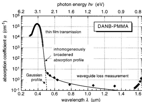
Fig. 3. Ultraviolet-visible-near-infrared absorption spectrum of DANB-PMMA. Open circles, data measured by transmission spectroscopy of an unpoled thin film (thickness  $0.6 \mu\text{m}$ ); filled diamonds, data measured in a planar waveguide (thickness,  $1.6 \mu\text{m}$ ). Curves, same meaning as for Fig. 2.
