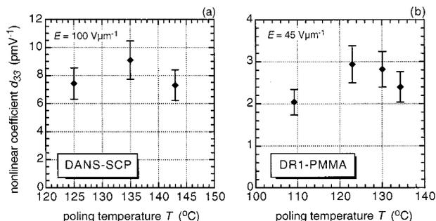
Fig. 8. Dependence of nonlinear-optical coefficient  $d_{33}$  on poling temperature for DANS-SCP and DR1-PMMA.
