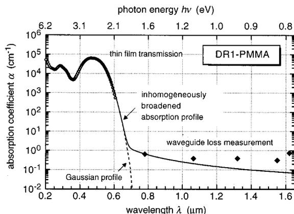
Fig. 4. Ultraviolet-visible-near-infrared absorption spectrum of DR1-PMMA. Open circles, data measured by transmission spectroscopy of an unpoled thin film (thickness,  $1.1 \mu\text{m}$ ); filled diamonds, data measured in a planar waveguide (thickness,  $1.5 \mu\text{m}$ ). Curves, same meaning as for Fig. 2.
