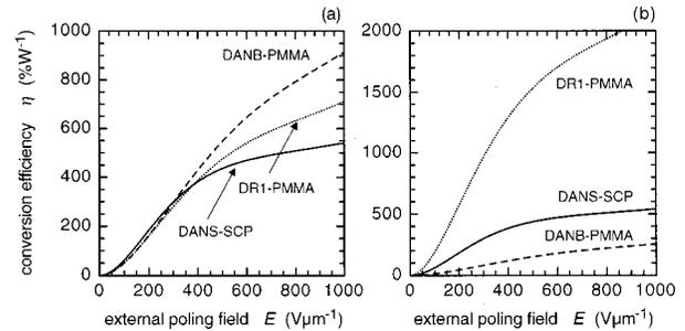
Fig. 11. Calculated normalized second-harmonic conversion efficiency  $\eta$  as a function of external poling field  $E$ . (a) Calculated for the actual chromophore loading; (b) chromophore number density assumed to be  $N = 1.3 \times 10^{27} \text{ m}^{-3}$  for all three polymers. The guide parameters are identical to those in Fig. 9.
