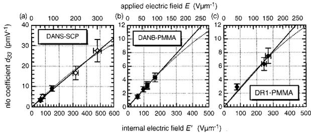
Fig. 7. Poling field dependence of the nonlinear-optical coefficient  $d_{33}$  for DANS-SCP, DANB-PMMA, and DR1-PMMA. The respective poling temperatures were 135, 100, and 120 °C. Dotted curves, fits according to Eq. (2); solid curves fits according to expression (7). (a) Solid and open diamonds, data from parallel-plate and in-plane poled samples, respectively. (b), (c) All data measured on parallel-plate poled samples.
