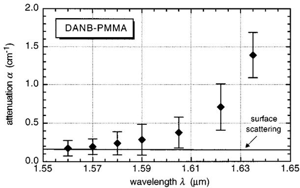
Fig. 5. Attenuation coefficient  $\alpha$  of a 1.5- $\mu\text{m}$  thick unpoled planar DANB-PMMA waveguide measured at 1.55–1.65- $\mu\text{m}$  wavelengths. Solid line, calculated surface scattering loss.
