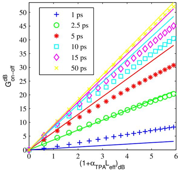
FIG. 3 On-Off gain  $G_{\text{on-off}}$ , plotted as a function of  $(1 + \alpha_{\text{TPA}} L_{\text{eff}})_{\text{dB}}$  for different pulse durations. Markers represent the numerical data obtained by solving equations (17) and (18), taking into account TPA, XPA, linear absorption and SRS. Solid lines correspond to the analytical formula.
