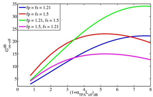
FIG. 9 Calculated on-off Raman gain  $G_{\text{on-off}}$  given by Eq. (21) as a function of  $(1 + \alpha_{\text{TPA}} L_{\text{eff}})_{\text{dB}}$  for different localization situations and taking into account the theoretical SPM-broadening of the pump pulse. The local field factors for pump and signal are set equal to 1.21 or 1.5, corresponding to a group velocity equal to  $c/5$  and  $c/8$ , respectively.
