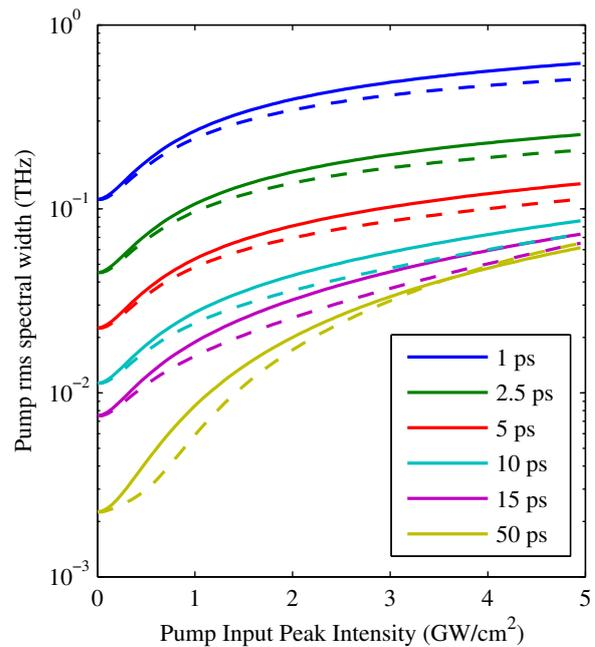
FIG. 6 The rms spectral width  $\Delta\omega_\sigma$  plotted as a function of peak intensity of input pump pulses of different pulse durations. The dashed curves show the output spectrum widths obtained numerically using Eqs. (3) (without considering pump depletion through SRS) whereas solid lines correspond to Eq. (33).
