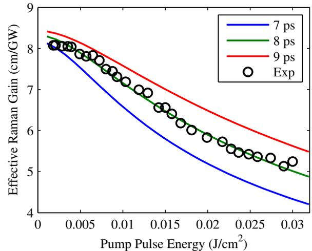
FIG. 8 Effective Raman gain  $g_R^{\text{eff}}$  plotted for several pulse durations as a function of pump pulse energy at the input of the waveguide. The solid lines show the analytical result using Eq. (15) and the circles correspond to the experimental data in Ref. [5].
