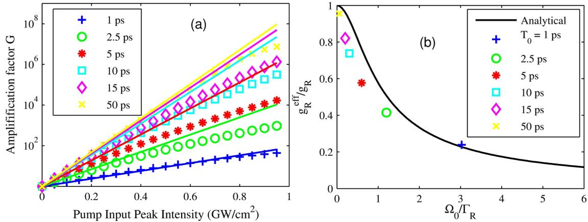
FIG. 2 (a) Amplification factor as a function of peak intensity  $I_p(0)$  for several pump pulse durations. Symbols show the numerical data obtained by solving Eq. (9). Solid lines correspond to the analytical formula (16). (b) Reduction in the Raman gain,  $g_R^{\text{eff}}/g_R$ , as a function of  $\Omega_0/\Gamma_R$  calculated using Eq. (15) with  $g_R = 8.9$  cm/GW. Symbols are obtained using numerical data in part (a).
