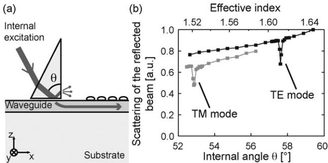
**Fig. 1.** (a) Coupling setup used for the internal excitation of labelled oligomers at the microarray surface. Light not coupled into the guide scatters at the unpolished prism face. (b) Typical measurement of scattered uncoupled light as a function of internal angle  $\theta$ . Dips correspond to guided modes (effective indices  $n_{eff}^{TE} = 1.61$  and  $n_{eff}^{TM} = 1.52$ ).
