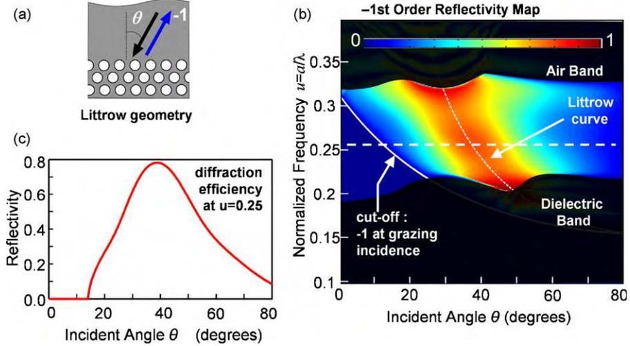
Fig. 3. (a) Littrow diffraction onto a PhC cladding; (b) color map of diffraction efficiency in  $-1$  reflected order, with cut-off curve and Littrow curve for a typical PhC; (c) plot of efficiency for the normalized frequency  $u = a/\lambda = 0.25$ . (For interpretation of the references to color in this figure legend, the reader is referred to the web version of the article.)
