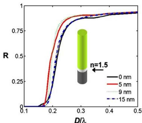
Fig. 3. (Color online)  $HE_{11}$  modal reflectance of facets connecting with a silver post (inset) for several values of the adlayer ( $n=1.5$ ) thickness  $t=0, 5, 9,$  and  $15$  nm ( $\lambda=950$  nm).
