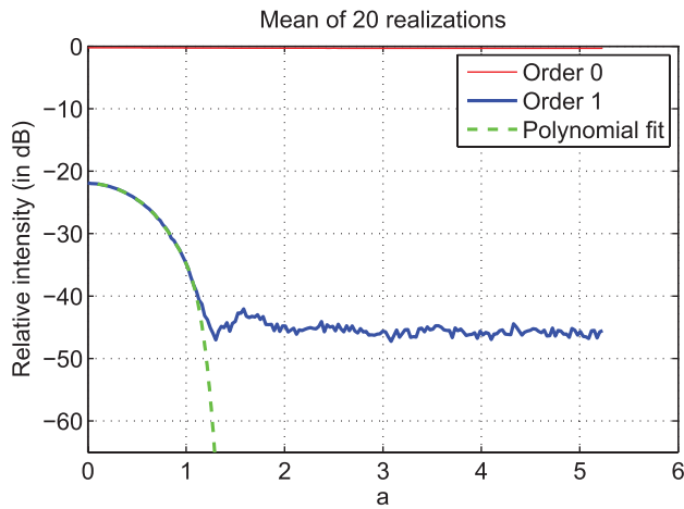
Fig. 9. (Color online) Evolution of the relative intensities of the order 0 and of the order 1 as a function of the parameter a for a pixelated lens of focal length f = 2 m encoded on a Voronoi SLM. Average of the efficiencies on 20 realizations of two-dimensional Voronoi components.
