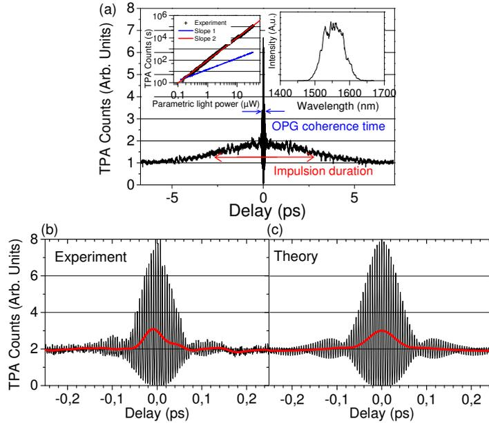
Fig. 2. (a) DSOC spectrum, i.e., variation of the TPA photocounts as a function of the delay  $\tau$ , of the TPA Michelson set-up of Fig. 1. The left inset shows the number of photoelectron counts as a function of the incident power. The quadratic behaviour clearly indicates a TPA process with an OPG in high gain regime. The right inset shows the spectrum of the degenerate OPG.
