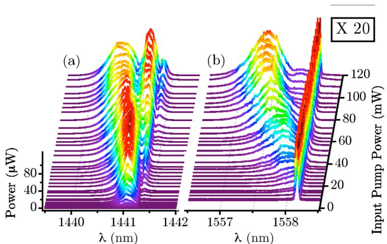
**Fig. 1.** Output spectra of (a) the pump pulses and (b) the amplified probe pulses measured for input average pump powers varying from 10 mW to 120 mW (the probe spectra are magnified by a factor 20). The spectral resolution is 0.01 nm.
