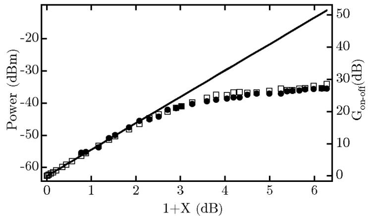
**Fig. 2.** Average power of the Raman amplified output signal in dBm with the corresponding on-off Raman gain (right axis) versus the parameter  $1+X$  in dB (filled circles). The values directly calculated from the measured lineshape of the pump spectra are plotted with open squares. The solid line corresponds to the un-broadened pump case.
