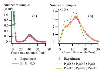
FIG. 4 (color online). Histograms in the collisional blockade regime (a) and in the intermediate regime (b). Fits of these results give the probability  $P_n$  of trapping *n* atoms. The dash curve obtained with  $P_2 = 0$  is unable to fit the experimental points in the intermediate regime.
