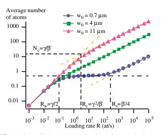
FIG. 1 (color online). Average number of atoms in the trap as a function of the loading rate R for different values of the waist.  $w_0 = 11 \ \mu m$  corresponds to a standard configuration. For  $w_0 = 0.7 \ \mu m$ , the blockade regime is clearly seen.
