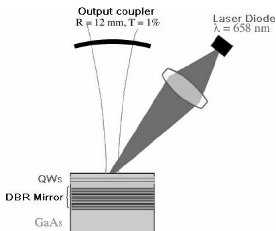
Fig. 7: Scheme of the VECSEL compact cavity
