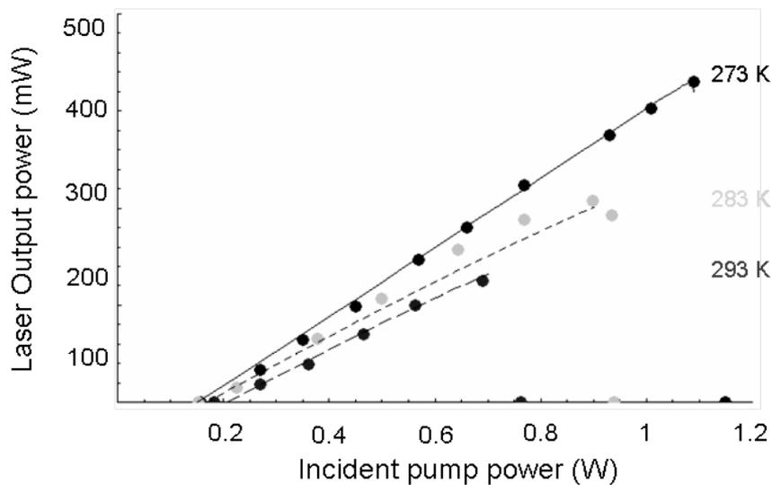
Fig. 6. Output power for different temperatures of the substrate  $T_{sub}= 273$  K, 283 K and  $T = 293$  K vs. the incident pump power on the semiconductor structure: Experiment (dots) and simulation (solid and dashed lines)
