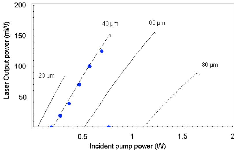
Fig. 5. Output power for different pump radii from  $20 \mu\text{m}$  to  $80 \mu\text{m}$  vs. the incident pump power on the semiconductor structure at room temperature (293 K): Experiment (dots) and simulations (solid and dashed lines)
