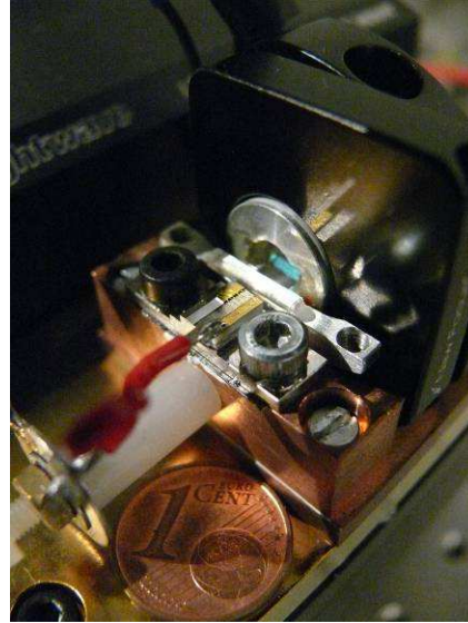
Fig. 6: Photograph of the laser cavity
